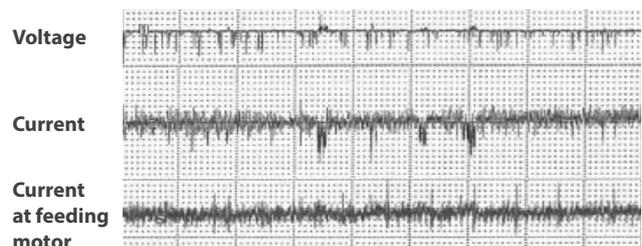
Electroplated welding wire enhances stable power characteristics during the welding process.
