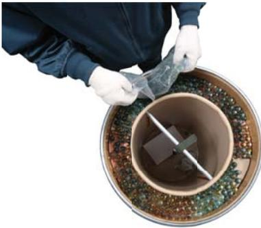
2. Remove the one-touch elastic band, steel bar, and pads.
