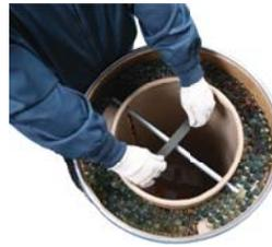
*Removing the steel bar and pads*
