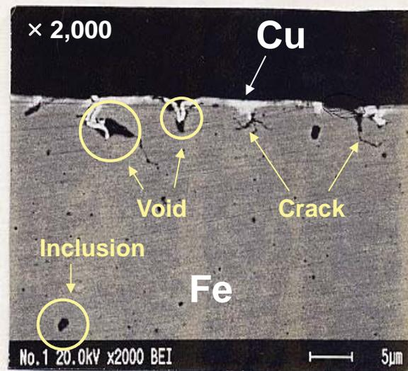
The electroplating process forms a consistent copper coating with a smooth finish over the surface of the welding wire. All of the wire strand's voids and cracks are filled with copper to create a welding wire that provides a consistent welding experience.
