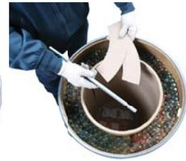
3. Pull the end of the wire through the feeding hole at the top of the cap.
